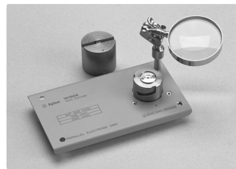
Figure 9. Agilent 16196B parallel electrode SMD test fixture
