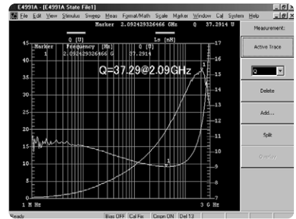
Figure 1. Ls-Q characteristics of a chip inductor
